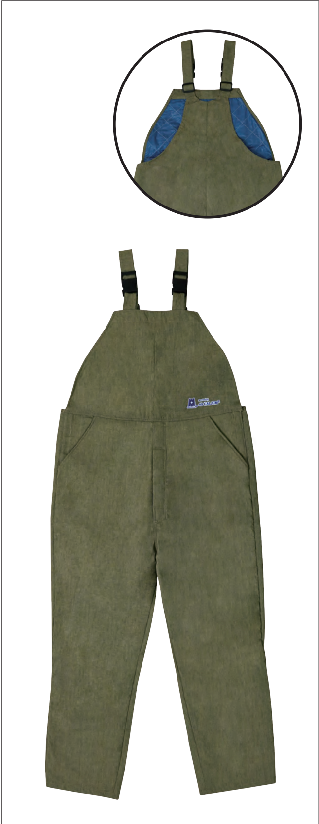
Arc Flash Bib Overalls FR hook & loop fastener Aramid sewing threads Expandable leg opening to fit over boots ASTM F1959 ATPV = 40 cal/cm² NFPA 70E PPE CAT 4 AR3
