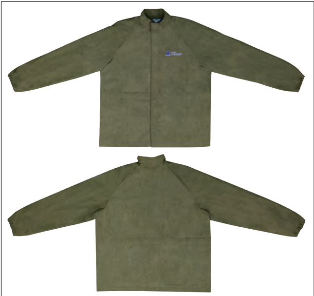
Arc Flash Jacket FR hook & loop fastener Aramid sewing threads Elastic waistband ASTM F1959 ATPV = 40 cal/cm² NFPA 70E PPE CAT 4 AR2
