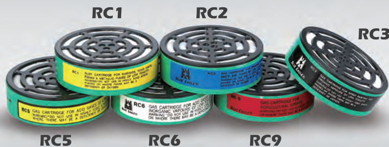
Cartridges RC1 : For dust RC2 : For organic vapours (with boiling point > 65 °C), mists of low toxicity RC3 : For Spray painting and organic vapours (with boiling point > 65 °C) of low toxicity RC5 : For sulphur dioxide and acid gases of low toxicity RC6 : For organic vapours (with boiling point > 65 °C), acid gases, and inorganic gases (such as chlorine Cl 2 and hydrogen sulphide H 2 S) of low toxicity RC9 : For agricultural sprays
