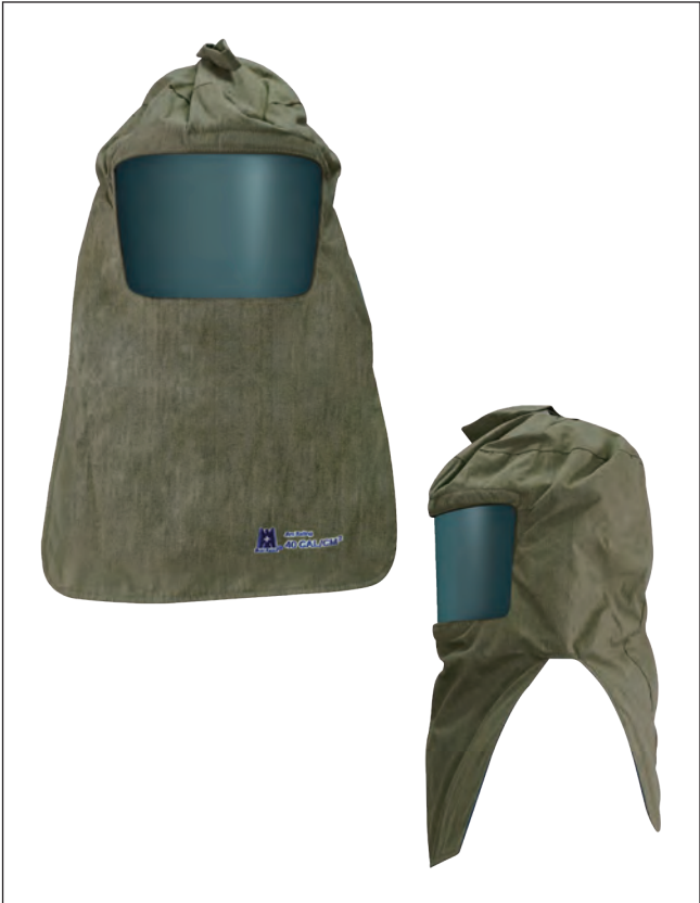
Arc Flash Hood Large field-of-view ANSI Z89.1 class E safety helmet ASTM F2178 ATPV = 40 cal/cm² NFPA 70E PPE CAT 4 ANSI Z87.1 – U6 R10 AR1
