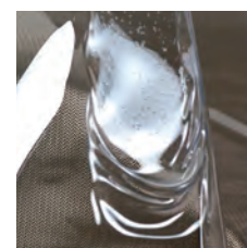
A clear visor molten by radiant heat
